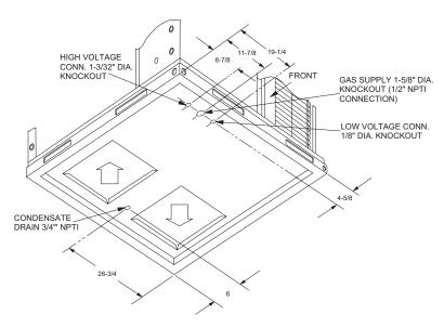
FIGURE 8 - UNIT DIMENSIONS - FRONT & BOTTOM
